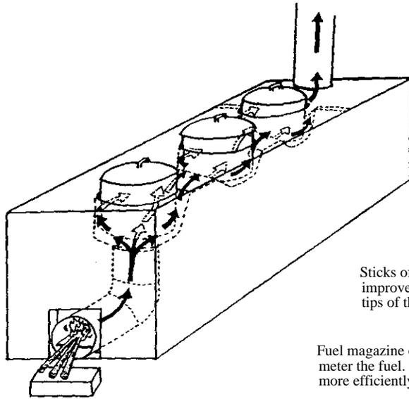
Rocket chimney increases draft. Smoke is drawn through flame and combusts.
