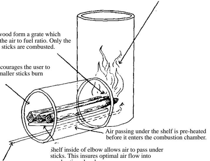
Air passing under the shelf is pre-heated before it enters the combustion chamber.
