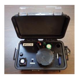
Function: Portable device for logging CO and PM concentration
