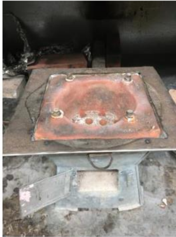
Figure 12 Final stove configuration, detail of 22 mm pot supports
